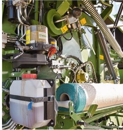
A chain lubricator and an automatic lubrication system are standard specification.
