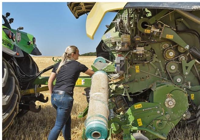
Rolls inside the chute make it easy to feed the new net roll into its cradle.
