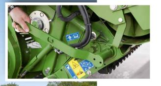
**Standard feature: manual blade group control** The standard manual control is a long lever that takes little effort to operate. This way you can quickly adjust the number of blades to varying conditions and customer needs.
