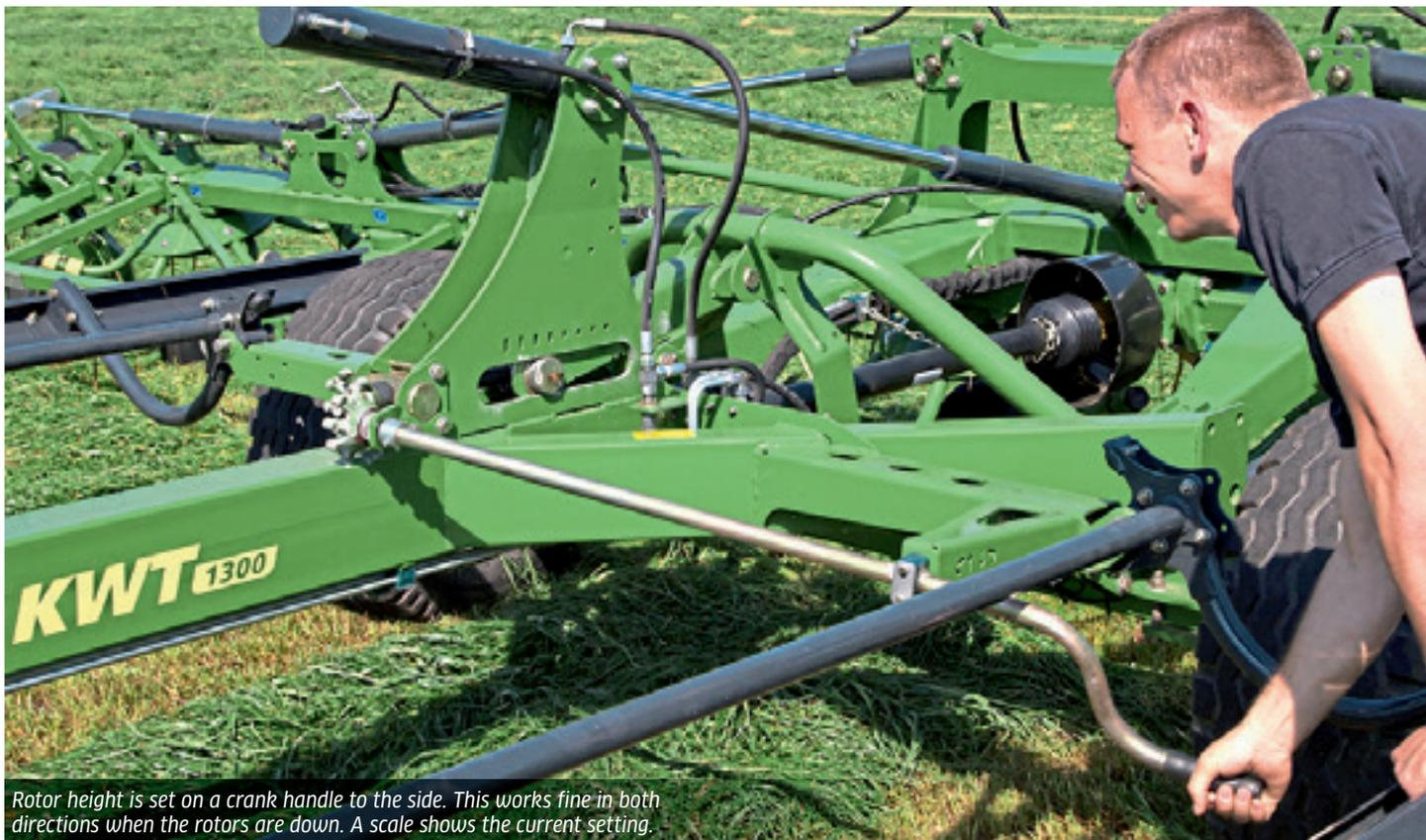
Rotor height is set on a crank handle to the side. This works fine in both directions when the rotors are down. A scale shows the current setting.
