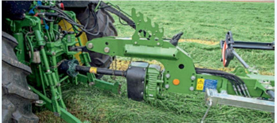
*Our German spec machine had a top mount hitch, but this can be repositioned for lower mounting. A headstock for coupling to the lift arms is an option.*
