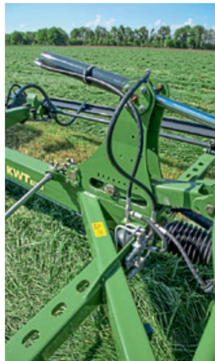
*Oil is directed to the nitrogen accumulator by the lift ram. When the accumulator is filled, the transport running gear is suspended by the rams which shifts the weight to the rotor wheels.*
