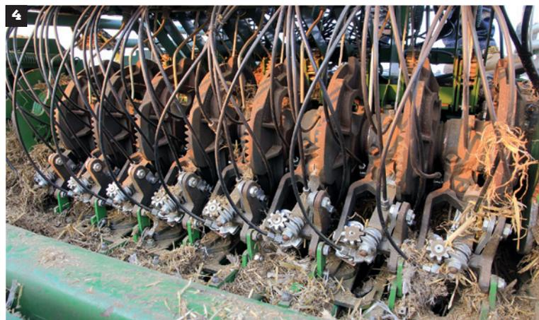
**1** The twine boxes are lowered hydraulically for easy filling and maintenance. **2** The machine can store enough twine to tie up to 800 bales. **3** The optional knottor fan keeps the twine feed system clear of chaff. **4** The eight double knotters are cleaned by blasts of air from an on-board optional compressor which operates independently of the tractor's air brake system.
