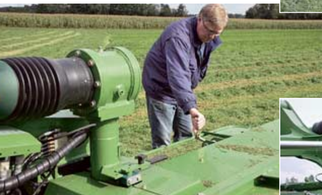
Conditioner intensity is set via a mechanical gearbox and on a crank lever that adjusts the baffle plate (left). Cutting height is altered hydraulically (below).
