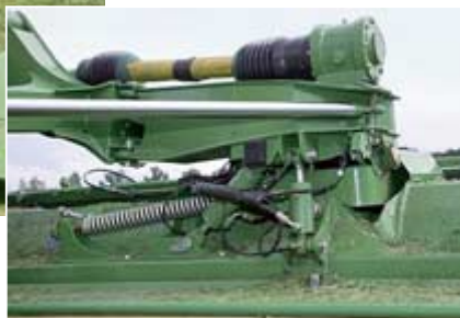
Conditioner intensity is set via a mechanical gearbox and on a crank lever that adjusts the baffle plate (left). Cutting height is altered hydraulically (below).
