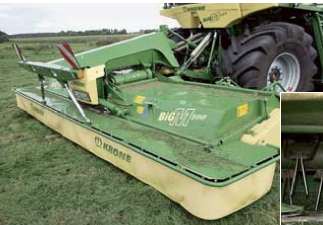
The 5.3m wide front mower unit comprises two individual cutterbars that work alongside each other.
