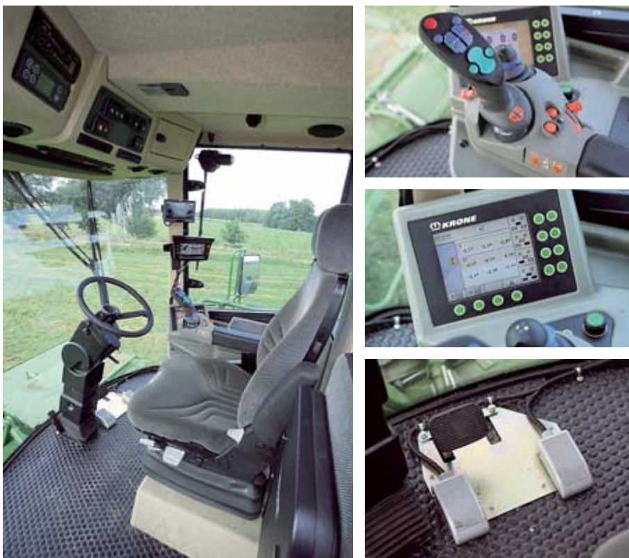
Cab hails from Krone's BiG X forage harvester. The Fendt-sourced joystick (top) continues to irk, although this unit is countered by the informative monitor (middle). The pedals (bottom) control the X's rear wheel position.
