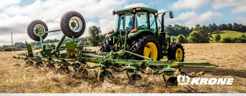
The Krone range of rotary tedders provides dependable machines in a full range of sizes and configurations. These machines not only deliver a superior quality of work and a high level of standard specifications, but also include several innovative features such as the maintenance-free OctoLink<sup>™</sup> finger clutches and liquid grease rotor drives.
