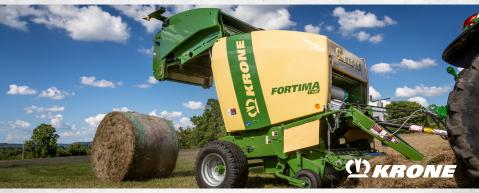
Krone's Fortima models produce 4' x 3'3" to 4' x 6' round bales. Smaller bale sizes are often preferred in grass silage, while larger diameter bales are preferred in hay and straw. The variable chamber allows producers the flexibility to adjust the bale size depending on the crop. Whether you are baling dry hay, baleage or both, the Fortima is a good fit for you.
