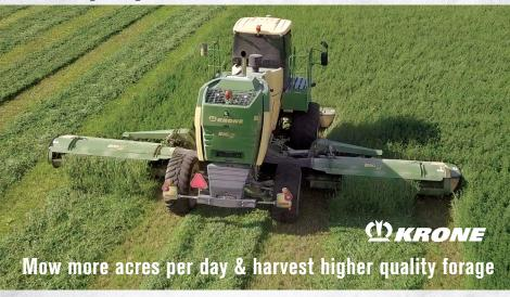
Mow up to 45 acres per hour and create 3 equal-sized windrows for fast dry down, with the BiG M 450 Mower Conditioner. Cutting widths from 29'6" to 36'9". Select the conditioner option to match your crops.
