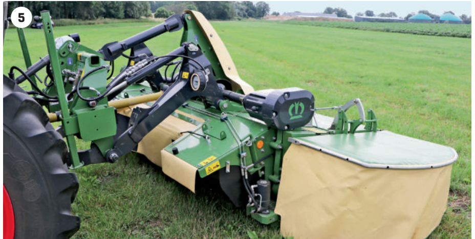
5 The EasyCut F 400 CV Fold is attached to a headstock with an integral lifting mechanism and has hydro-pneumatic suspension.
