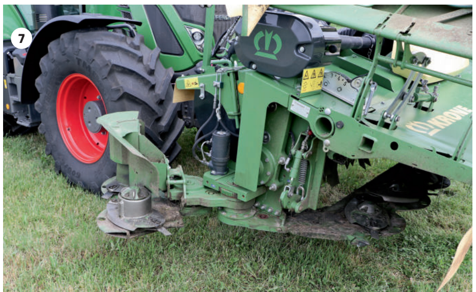
7 The outer elements of the mower bed swing backwards on a slewing ring. The solution maintains the position and timing of the discs so that you can cut at a width of 4.04 metres and still have a transport width of less 3.00 metres.
