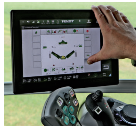
The Comfort control system requires an ISOBUS terminal and an ISOBUS joystick. We used the tractor's ISOBUS-compatible terminal.
