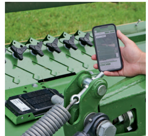
The SmartConnect Solar is a digital vibration data logger which is used for implementing telemetry on attachments.
