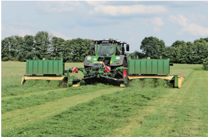
With the belts up and out of work, the mowers produce three full-width swaths.
