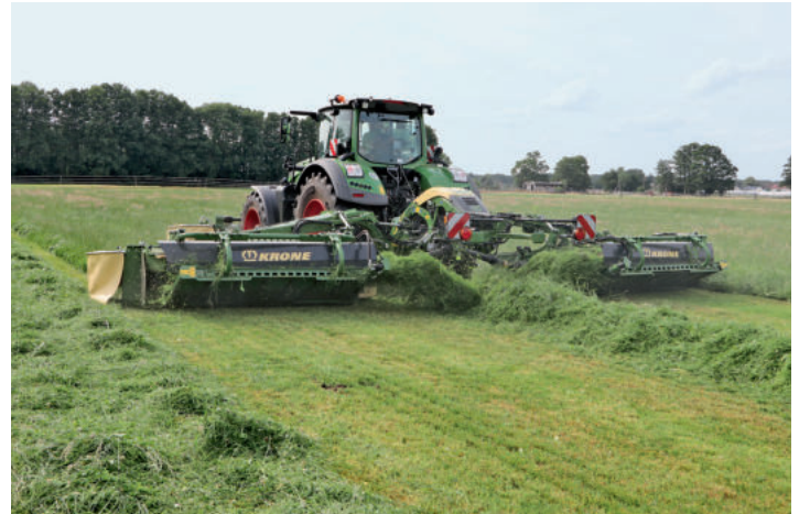
Compact swaths are produced by varying the belt speed.
