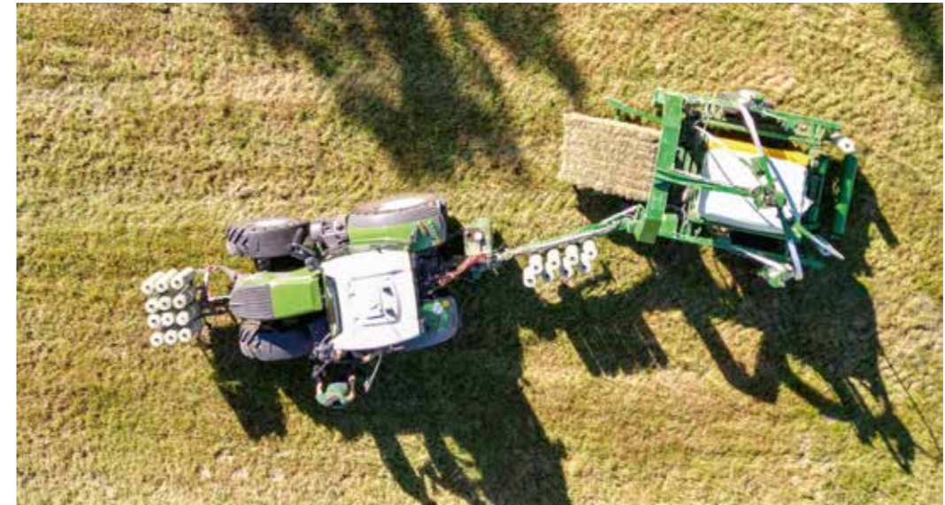
The wrapper pivots to the right to pick up the square bales for wrapping.
