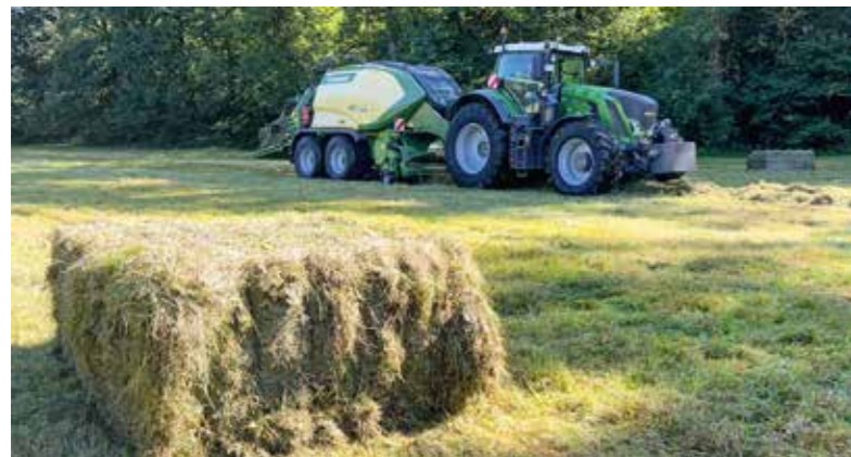
Packed to higher densities at larger volumes, square bales contain considerably more material. As a result, baling and wrapping costs per tonne are lower.
