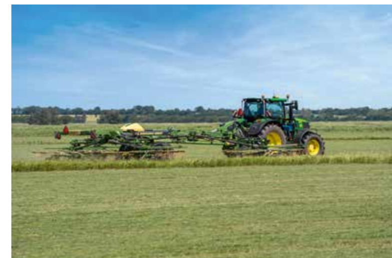
By using CTF to forage harvest, enormous harvesting yields of up to 25 ha per hour are achieved as a working width of more than 20 m is placed in one swath.
