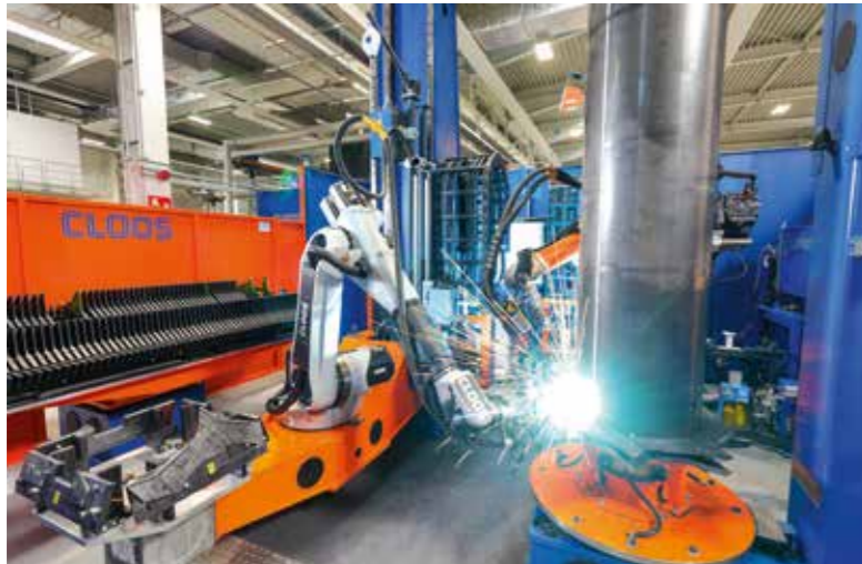
Pure precision when the robots weld the rotor shafts of the loading and forage transport wagons. The highlight of automated production is an automated quality assurance process and self-learning total system.
