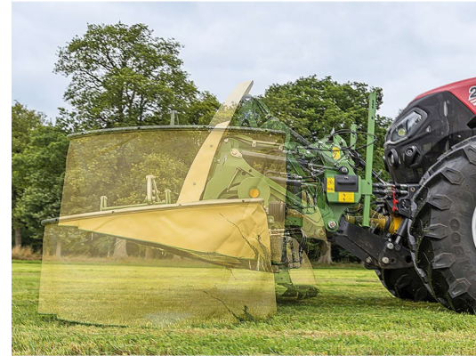
The suspension system is worked by a single-acting spool, which also lifts the mower at the headland. It's an effective set-up.
