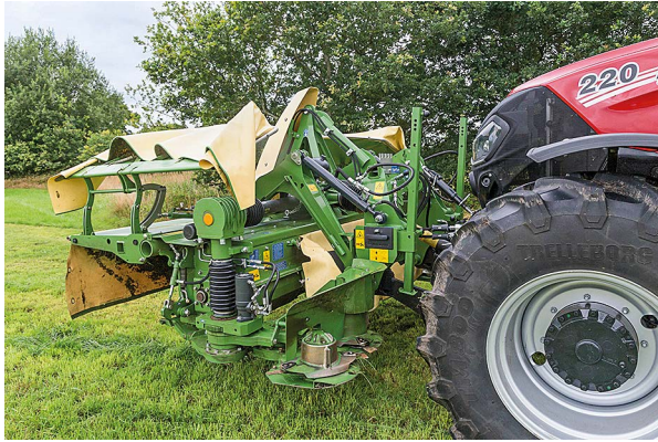
The two outer discs swing backwards hydraulically, the side guards automatically folding upwards. Convenient.
