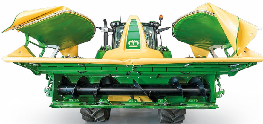
A new feature, not shown on the preview machine at the last Agritechnica, is a swathing auger for grouping 4.0m of cut grass into a row that fits between the tractor wheels.
