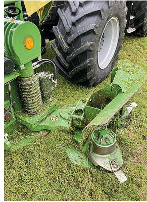
A hydraulic motor powers a sprocket to slew the wing into its different positions.
