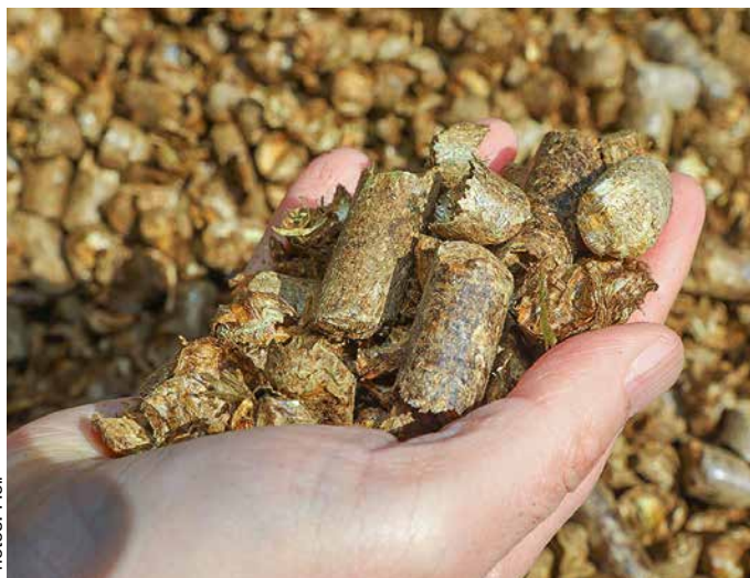
◁ The pellets are a bit crumbly. This is because Bernd Pommerehne operates the pellet harvester at maximum throughput rates. But that's not a problem in the digester.
