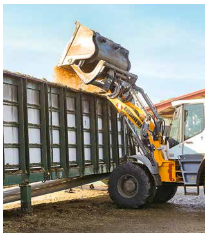
△ No special equipment is needed to add straw pellets to the substrate mix; they are simply tipped into the feed unit.
