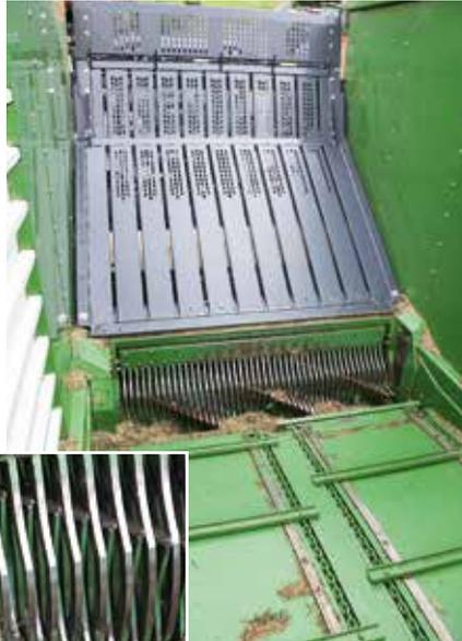
The headboard can now pivot, and the new rotor, along with the stripper fingers, is made from Hardox steel.
