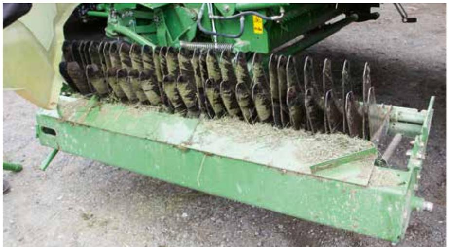
A total of 46 knives offer a 37mm chop length, and the blade bank pulls out to the side for convenient service/maintenance access. The Speed Sharp sharpener system will be available from 2018.
