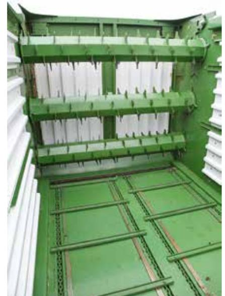
Chain/slat floor has four round steel chains and is powered by a pair of hydraulic motors with fast advance mode. GD models come with two rear beaters, but the majority of UK/Irish machines will be GL versions with no beaters.
